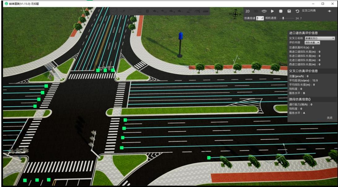
(12) “连接车道到路段”功能
